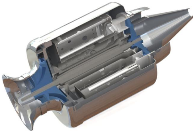
Figure 2. The model of KJ 66 engine in FloEFD.
