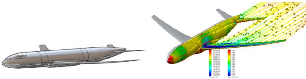
FIGURE 3. WBT0 CAD model (left) and the pressure distribution with flow trajectories colored by Mach number at angle of attack 4^\circ (right).
